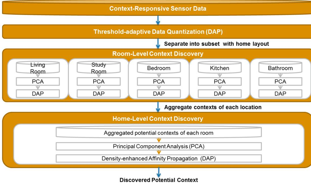
Fig. 1. System Architecture of M2M-based Anticipatory Reasoning for Contexts.
