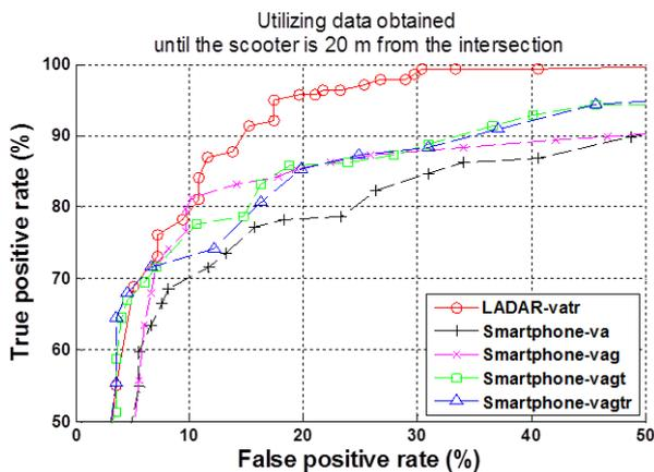
Figure 2. Receiver operating characteristics of our prediction algorithm. (v: GPS velocity; a: GPS acceleration; g: G-sensor acceleration; t: time to red light estimation; r: traffic signal status)
