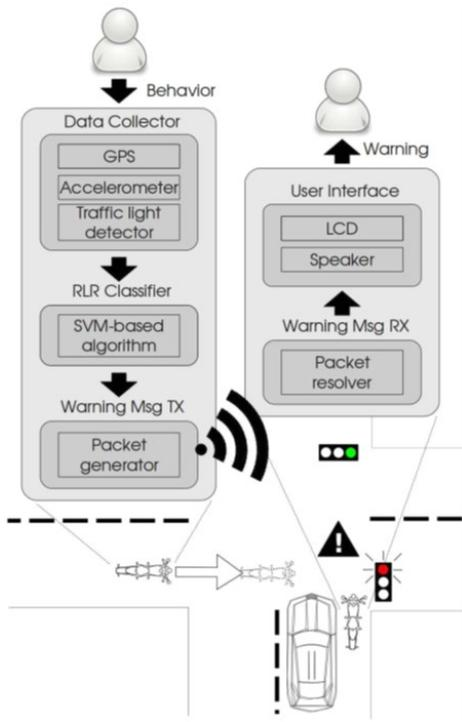
Figure 1. The system block diagram of our collision avoidance system
