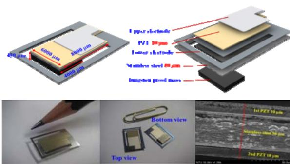
Figure 1: Paper clip sized energy harvesting device
