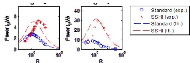
Figure 2: Power enhancing experiment with  $k^2Q_M = 0.17$  and  $0.39$
